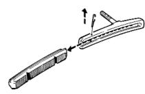
**2.** Slide the new brake pad in ALL THE WAY until it is fully aligned with the forward edge of the brake pad holder. Push the locking pin in until it is fully engaged.
