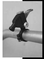
Slide or mount the complete remote lever onto the handlebar.
