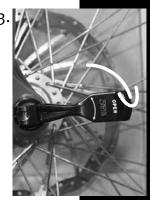
On Thor: Insert the supplied aluminium plug into the hole just above the right drop out when using the Maxle 360°.
