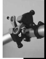
The lever with the black aluminium dot (1) without snap actuates Flightcontrol Remote FCR. It is only actuated for a short time and snaps back again when releasing.
