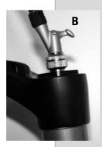
**Attention:** Activate the Flight Control Remote lever several times during pumping, to equal the air pressure in the main and negative air chamber!
