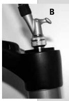
**Tip:** don't screw the pump head too tight onto the valve, otherwise it will be difficult to flip the lever to position B.
