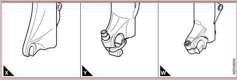
Picture 4 - Wheel axle securing systems: (X) standard fork dropout, (Y) QR20 Plus "with bolt", (W) Ø 20 mm through hole axle
