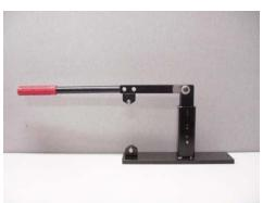
H - Rear Shock Compression Test Fixture
