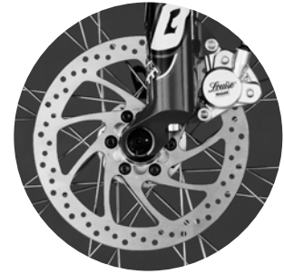
Brake caliper and rotor MAGURA Louise®
