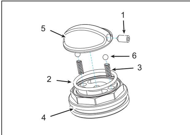
Lefty MAX rebound adjuster assembly (exploded view)
