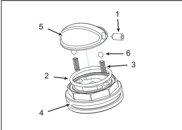
Lefty MAX rebound adjuster assembly (exploded view)
