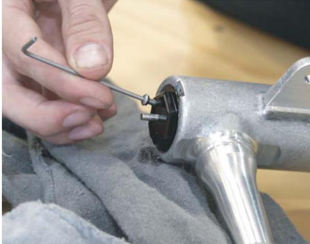
5. Use a 22mm socket to carefully remove the lower cap. Hold the bottom of the fork up when removing the cap. Once unthreaded, slowly pull up on the cap to remove the compression damper.
