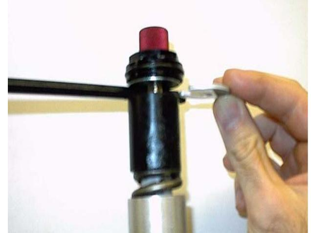
The shims are located between the top washer and preload spacer. Refer to "Illustrations" starting on page 20.
