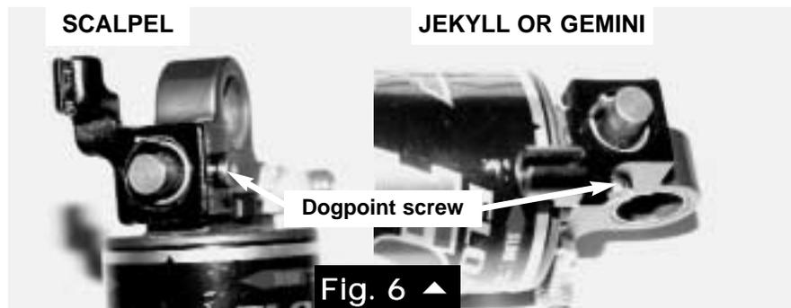
4. Now choose a lockout cam set screw position. If your cable stop bracket faces away from the shock body (Scalpel), thread the cam set screw into the position on the small radius of the cam. If the cable stop faces towards the shock body (Jekyll and Gemini),
