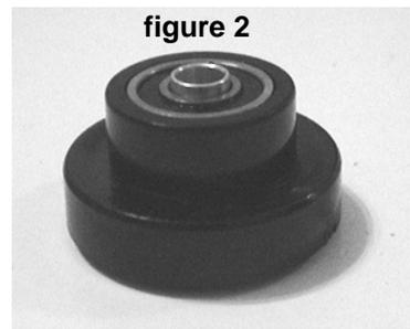
**6)** Press the second R4-2RS bearing into the other side of the flip-flop roller. Take your time on this step. This will encapsulate the roller axle inside the roller, between the two bearings. See **figure 2** for illustration of correct final installation.
