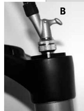
**Tip:** don't screw the pump head too tight onto the valve, otherwise it will be difficult to flip the lever to position B.
