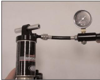
only the air left in the pump itself and not from the shock. This does not affect your pressure setting in the shock. Likewise, when you install the pump, the shock will fill the pump and reduces the registered pressure previously installed in the shock. This usually is a 10-15 psi difference
