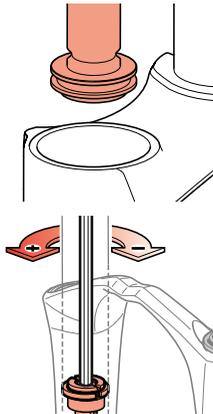
**Rebound adjustment by internal adjuster - Right leg**
