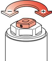
**Spring preload by external adjuster - Both legs**
