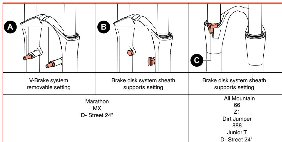
Picture 3 - Braking system settings
