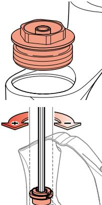
**Rebound adjustment by internal adjuster - Right leg**
