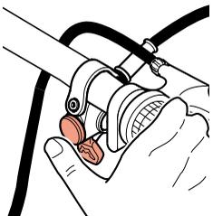
By pulling the control lever, the hydraulic configuration of the fork changes allowing the rider to obtain the best setting for climbing (the same as the "CL" position of the TST cartridge), regardless of the position of the adjustment knob on the fork.
