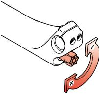
By turning the adjuster clockwise, you increase the hydraulic damping making the fork slower during the rebound phase.
