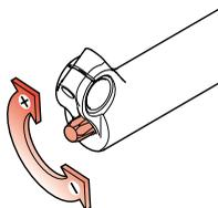
**Compression adjustment by external adjuster - Left leg
