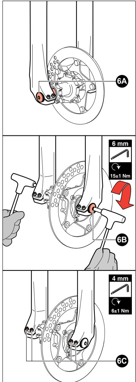
**Picture 6 - Wheel Installation on 66 end 888 series forks**
