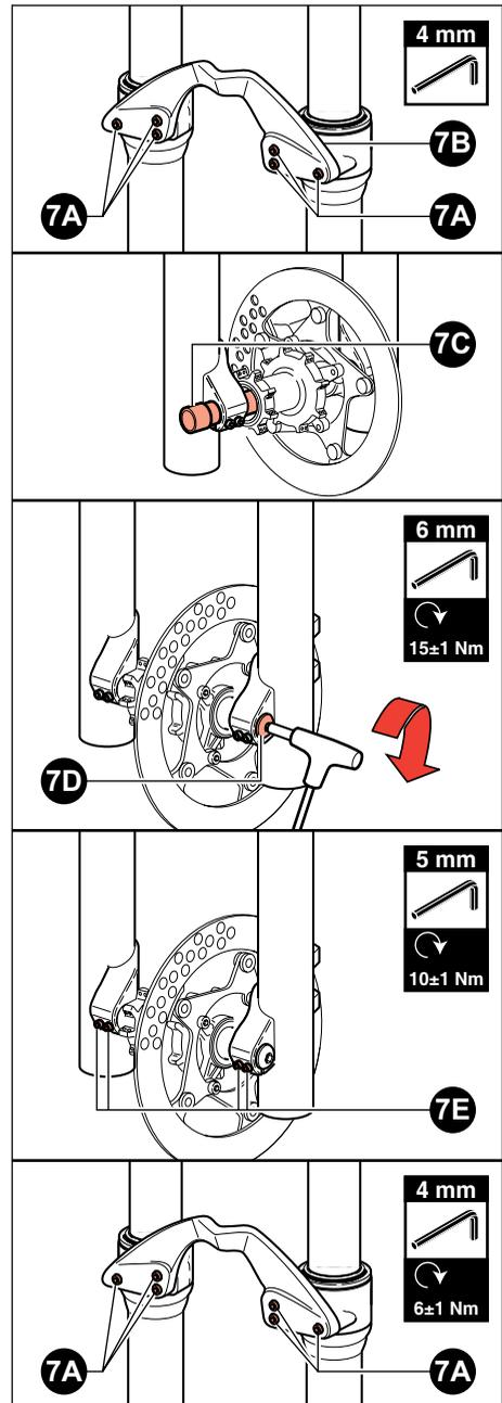
Picture 7 - Wheel Installation On Monster Series Forks
