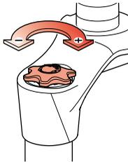
By turning the adjuster clockwise, you increase the hydraulic damping making the fork slower during the rebound phase.
