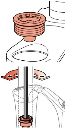
Using a small pin extractor eliminate any pressure from the right leg.
