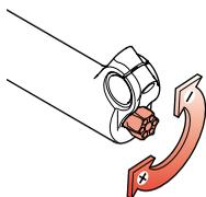
**Compression adjustment by external adjuster – RC2
