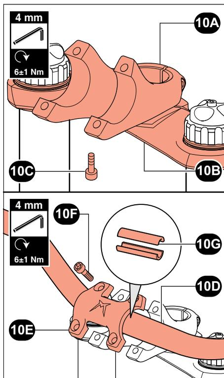
**Picture 10 - Handlebar Clamp Installation For The 888 Series**
