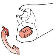
**Compression adjustment by external adjuster - Left leg (Not present in the version with +ETA / + TAS option)**
