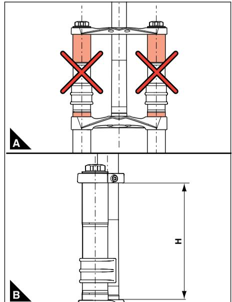
**Picture 2** - Dual crown forks installation on the frame: (2A) Crowns fastening, (2B) Steer tube maximum length between crowns
