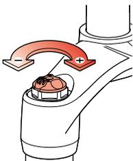
**Rebound adjustment by external adjuster – RC2 cartridge
