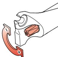
By turning the adjuster clockwise, you will reduce the maximum travel and the fork's length.
