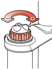
**Spring preload by external adjuster - Both legs (RC2X)**
