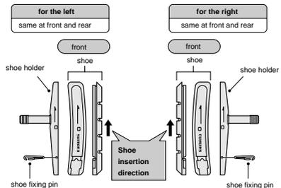
Insertion of shoe fixing pin is very critical to keep shoe properly fixed in place.
