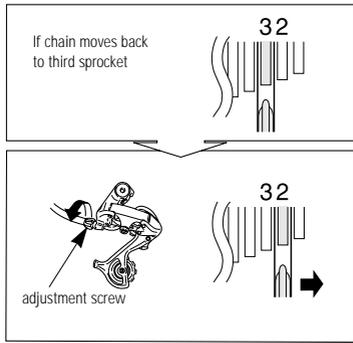
Turn the adjustment screw so far to the right until chain jumps back to second sprocket.
