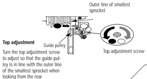
2. Drive the pedals forward a few times. In case of chain noise, adjust the derailleur with the adjusting screws.
