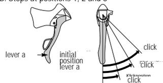
shift one gear to next bigger sprocket:
