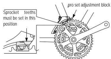
The derailleur must be adjusted as per illustration. The pro-set adjustment block may not be removed.
