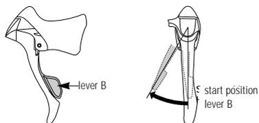
When lever b is operated, there is one click where trimming (the noise preventing mechanism) engages and a second stronger click when the gear change stroke is completed. After trimming, the next (light) push to the right will complete the gear change stroke to the smaller front chain-ring.
