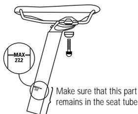
If you need to change the inclination of the saddle or the horizontal position, please make sure not to exceed the max. tightening torque.
