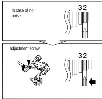
Loosen the screw so far to the left until chain touches the third sprocket.
