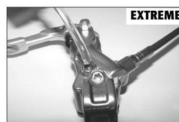
**⚠ WARNING! Before removing SYRINGE 2 from the pump, test the brake action a few times and press down on the brake itself to make sure that the diaphragm is in the correct position.**
