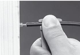
**5.** Press by hand a **new** insert into the hose until it is **fully seated**. Clamp the hose into the groove of the mounting device as shown...
