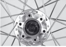
Use spokes with a diameter of 2 mm (arc)/ 1,8 mm which you cross three times.
