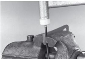
**6.** ...or clamp the mounting device as shown into a vice and hammer the insert **carefully** into the hose.
