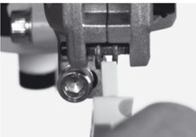
Check out whether the “finger” of the transport device fits in-between the “ears” of the brake pads. **On the picture on the left this is NOT the case, the pads must be changed!**
