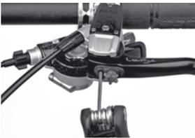
**10. Reach adjust is done with a 2,5 mm Allen key.** Turning key clockwise: lever blade moves away from the handlebar, turning counterclockwise: blade moves to the handlebar. On Louise models without BAT feature you find the reach adjust screw under the black dust cover of the lever blade.
