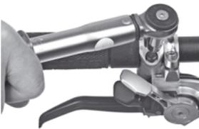
2. Mount the brake lever to the handlebar with a 5 mm allen key. **Tightening torque 4 Nm/ 34 in.lbs**
