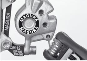
2. Remove the brake pad fitting screw with a 2mm allen key.
