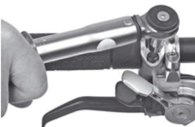
2. Loosen the brake lever clamping screw with a 5 mm allen key. Turn the brake lever and ensure that **the reservoir points approx. 15° upwards from the horizontal position.**
