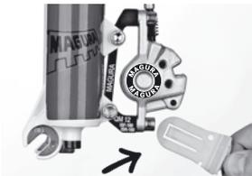
6. The transport device prevents the brake pads from being pushed out too far by unintended lever squeeze when the wheel is removed. It is impossible then to install the wheel with the rotor. So never throw away the transport device but keep it and always clip it between the brake pads as shown when the wheel is removed.
