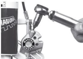
5. Fix the Heat Eater fitting of the caliper so that it points UPWARDS!. Unscrew now the bleed screw with a 5 mm allen key. Screw in the prepared syringe and tighten it with a 8 mm open end spanner.
