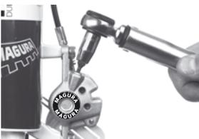
12. Remove the filling syringe and screw in the 5mm allen bleed screw. **Tightening torque: 2,5 Nm/ 22 in.lbs.** Re-install the brake pads and the wheel.
