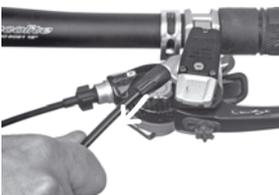
**8.** Always check for correct installation by pulling on the hose. Make sure that the system has no leaks. Squeeze the lever blade, hold pressure and check hose connections and the reservoir cover for eventual leaks.
