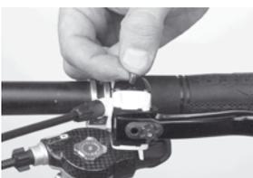
11. Close the plug on the reservoir cover as shown by pressing it by hand into the drill. That's it!
