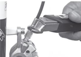
3. Tighten the prepared end of the new hose onto the Heat Eater.
