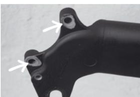
Make sure that the caliper fitting eyelets on your frame or fork are free of any paint, powder coating or burrs. (arrows). If this is not the case you should contact your dealer who is able to care for the absolutely necessary even surface with the help of the MAGURA Gnann-o-mat disc optimizer tool (also see page 10).
