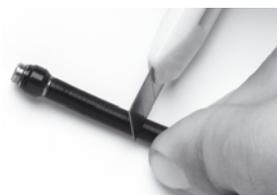
4. Put the hose on a workbench and shorten it with a sharp knife. The best tool is the MAGURA hose cutter. **Do not use saws or pliers!**
