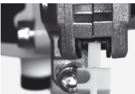
Here the “finger” of the transport device fits between the “ears” of the brake pads. **The pads are still o.k. Remember: The lever has to be pulled during this procedure. Use for this a rubber band or a cable tie.**
