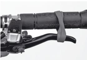
**If the bike is transported upside-down squeeze before the lever blade, hold pressure and fix the lever blade in this position with a rubber band or a cable tie as shown on the right photo.**
