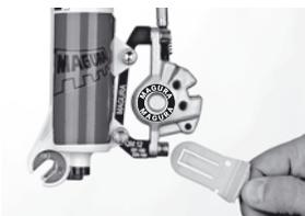
**Never throw away the transport device, which has been delivered with the brake. Always clip it between the brake pads whenever the wheel is removed (e.g. transport of the bike).**
