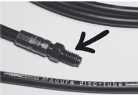
2. Prepare a new hose: Use only the reinforced MAGURA Disc Tube (wearing also this imprint). One end of this hose comes **with a pressed fitting with blue loctite threadlock**, which has to be screwed into the Heat Eater as described above. The hose is available with 0° and 90° fittings (c.f. page 20)
