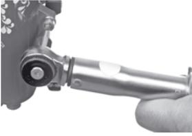
3. Mount the adaptor onto the fork or the frame. Use a 5 mm allen key. Please follow carefully the mounting instructions that come with the respective adaptor! If you use a thru-axle hub on the front you might have to use thicker 3 mm spacers (depending on fork model). These are available separately (code: 0720 829).
