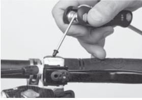
6. Remove **ONLY** the bleed plug of the reservoir with a 2,5mm Allen key that you insert into the plug before turning it slightly. The reservoir cover and the membrane underneath remain on the brake lever!
