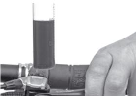
9. Actuate in addition **CAREFULLY** the lever blade to chase tiny air bubbles that might hide within the system. The job is done when no air bubbles can be seen after having followed the steps above several times.
