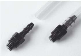
3. Prepare the transparent filler tube by pushing in by hand the M6 barbed fitting. Put the other end of the filler tube on the syringe and fill the syringe **completely** with MAGURA ROYAL BLOOD mineral oil. Fill the syringe completely and make sure that **there are no air bubbles inside.** Turn the syringe eventually to push out air bubbles.
