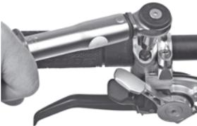
1. Loosen slightly the clamping screw of the brake lever with a 5mm allen key and **ensure that the reservoir points upwards approx. 15° from the horizontal position.** Slightly tighten the clamp screw in that position.
