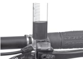
10. **Before you remove the syringe on the reservoir make sure that there is only a small quantity of oil inside.** Place a rag around the brake lever and the caliper thus preventing overflowing oil from dropping down and contaminating and killing the brake pads. Remove the syringe and close the end that was inserted into the reservoir quickly with your finger. Empty the remaining content of the syringe into a container.
