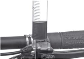
7. Put the second syringe of the service kit **WITHOUT PLUNGER** into the opened drill of the reservoir cover. Push oil from the brake caliper upwards until the oil column arrives in the syringe on the reservoir. You will see air bubbles now.
