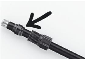
**7.** Slide on the sleeve nut and a **new** olive onto the hose. Push the hose with the sleeve nut and the new olive **fully** into the brake lever and tighten the sleeve nut with an 8 mm open-end wrench. **Tightening torque: 4 Nm/34 in.lbs.**
