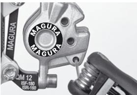
5. Secure the new pads with the fitting screw, a new one is delivered with the new pads. **Tightening torque: 1 Nm/ 9 in.lbs. Check the correct fitting of the pads by pulling them. The fitting bolt of the pads has to be correctly installed e.g. it has to go through the drills of the pad holders and then correctly screwed into the caliper.**
