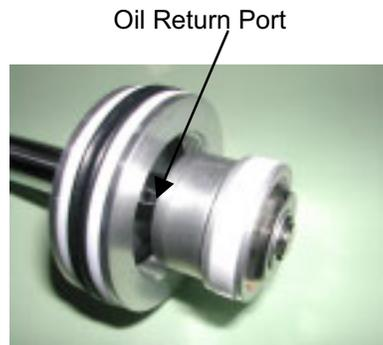
**NOTE:** Damping oil that would be in the bleed container is not shown in these steps to provide clarity.
