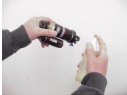
2. For leaks at the adjuster eyelet or damper end of the air canister, refer to the detailed disassembly instructions contained in the section on **DAMPING SYSTEM BLEEDING - Swinger Air**. This will guide you on how to replace the applicable o-rings and seals.
