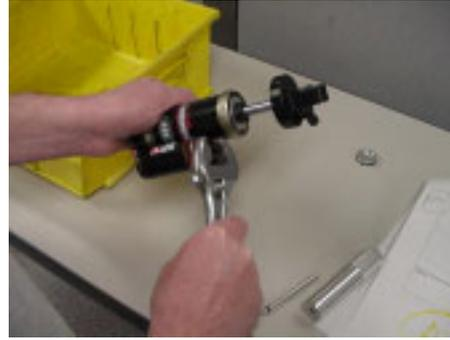
26. Clamp adjuster eyelet in soft jaws. Grease air canister threads, and screw canister onto eyelet. Tighten using strap wrench on canister.
