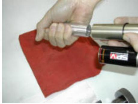
9. Change out o-rings and seals where indicated (#of o-rings/seals in each assembly noted in photo) and grease with a thick grease such as Motorex Bike Grease 2000
