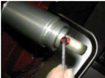
Schrader Removal Using 3mm Hex Wrench
