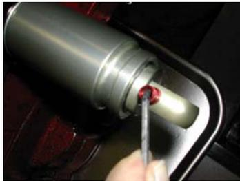
Schrader Removal Using 3mm Hex Wrench
