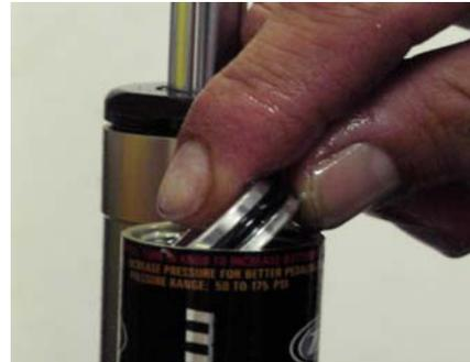
18. Back the IFP tool out fully as pictured. Using the IFP tool push the IFP piston fully into the reservoir. Screw the tool in hand tight until the flange is flush with the air reservoir body. Using a 6mm hex wrench, adjust the IFP Locating Tool so that the indicated travel matches the shock travel. Make sure that the travel indication line is flush to the top of the tool.
