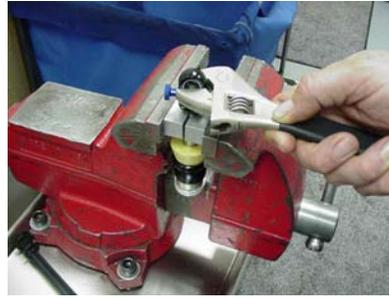
12. Using pliers, remove the rebound adjuster needle from end of the damper shaft.
