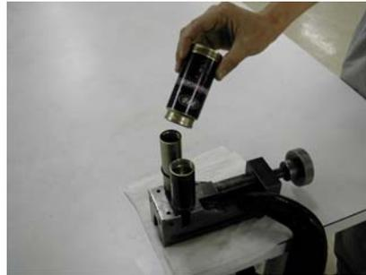
7. Remove air piston from canister
