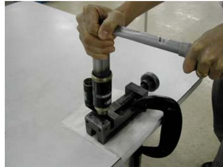
17. Top up the oil level in the reservoir. In a small container of oil tap the IFP to get the air out from under the o-ring. Insert the IFP into the reservoir starting at about a 45 degree angle so that you burp the air out of the piston cavity. Push the IFP past the threads in the reservoir. Only press the piston in just beyond the reservoir threads.
