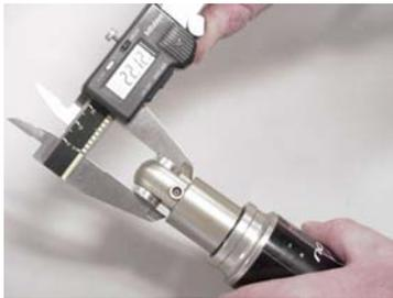
2. Measure mounting hole size. Current hardware is typically designed to accept a 6mm or 8mm fastener.
