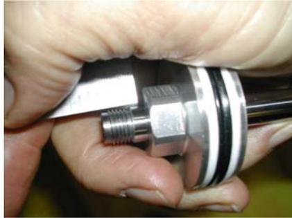
12. Insert the needle and o-ring into the damper shaft until they are firmly seated. Put on the bottom out bumper and then hand tighten the rebound damper eyelet.
