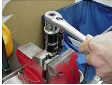
6. Remove the air canister.
