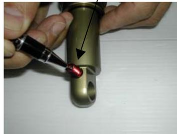
3. Remove hardware as shown under **HARDWARE REMOVAL**. Place adjuster eyelet in a vise using soft jaws. Using a rubber strap wrench to prevent damage, loosen the air canister completely. Pull back the air canister and slide it off the damper body to expose the 10mm damper shaft.
