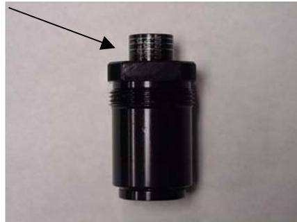
17. Install rebound adjuster needle, pointed end first. Push until the needle and o-ring seat firmly in the damper shaft.
