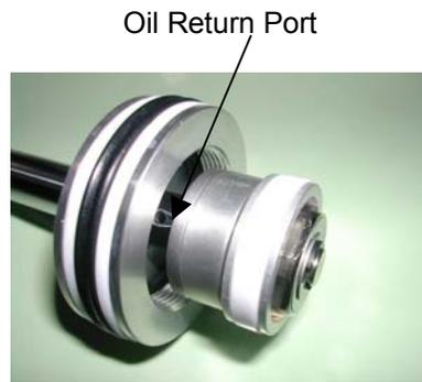
**NOTE: The following bleed procedures will work on all model years of the Swinger 4 way Air shocks.**
