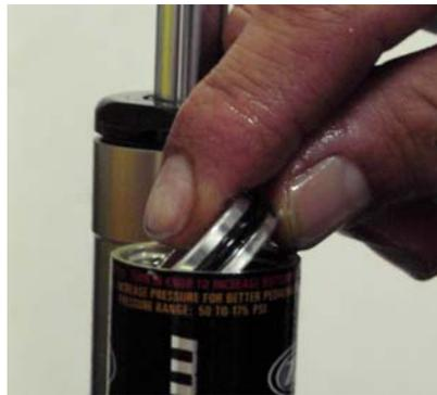
16. Back the IFP tool out fully as pictured, Using the IFP tool push the IFP piston fully into the reservoir. Screw the tool in hand tight until the flange is flush with the air reservoir body. Using a 6mm hex wrench, adjust the IFP Locating Tool so that the indicated travel matches the shock travel. Make sure that the travel indication line is flush to the top of the tool.
