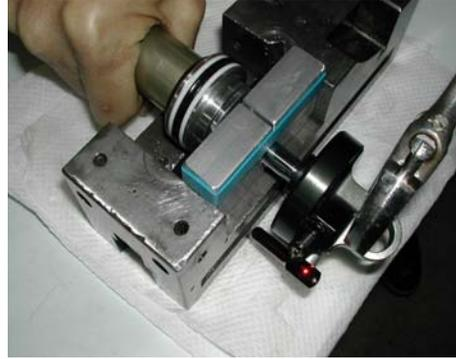
5. Clamp the damper body eyelet in a vise using soft jaws and remove the damper assembly by removing the air piston as shown. Remove from vise and drain damper oil into a container and discard.
