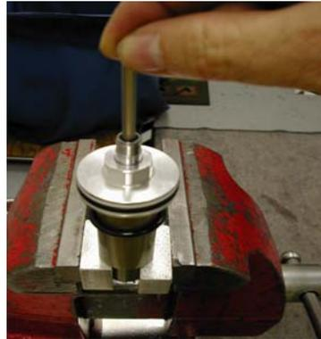
13. Remove the valve core from the Schrader valve and fully extend the damper shaft from the damper body. This will set the level of the IFP. Replace the valve core.
