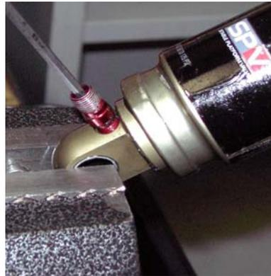
16. Clamp the adjuster eyelet in the soft jaw vise. Grease the air canister threads and screw the canister on to the eyelet. Tighten using strap wrench on canister to 13-21 in/lbs or 15-24 Kg/cm.
