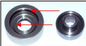
9. Pull apart the two pieces of the SPV valve, gently clean both the inside of the piston and the out side of the shim head to remove any oil or old grease that maybe on them. Check the quad seals for damage and replace if needed. Lightly grease the quad seals with Silicone grease and reassemble the valve and recheck for proper function. Set aside for reassembly.
