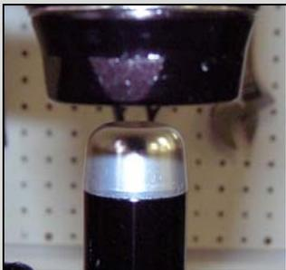
23. Insert the air can installation tool into the damper body. Slide the air can over the tool and on to the damper body. Next install the top out bumper then remove the Installation tool.
