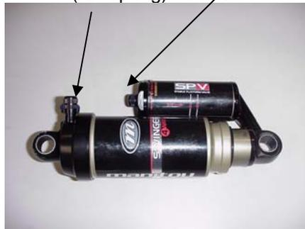
5. If when you pressurize the air canister the shock collapses to its shortest travel position, the shock has an air piston leak into the negative chamber. Place the shock in the shock tester and extend it to its full travel. Depress the adjuster eyelet Schrader while the shock is extended under load. If it remains in the full travel position, refer to the section on DAMPING SYSTEM BLEEDING - Swinger Air for instructions on servicing the air canister and piston seals.
