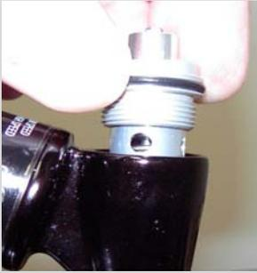
17. Secure the shock eyelet in a vise with the mounting hole for the intrinsic damper up. Fill the hole with oil and install the Intrinsic damping control unit. If it is an adjustable unit for an X6, be sure that the adjusters are turned out to the lowest settings.
