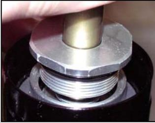
26. Insert the damper piston/shaft assembly into the damper body. Screw down the top cap and torque to 60-70inlbs.
