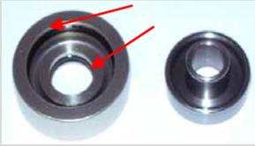
15. Pull apart the two pieces of the SPV valve, gently clean both the inside of the piston and the out side of the shim head to remove any oil or old grease that maybe on them. Lightly grease the quad seals with Silicone grease and reassemble the valve and recheck for proper function. Set aside for reassembly.
