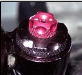
11. If you are servicing an ISX-6, remove the red and black knobs, use caution as the detent balls and springs are VERY small. Next remove the Intrinsic damping assembly by unscrewing it counter clock-wise. Pull the assembly out of the damper body. Do not disassembly the Intrinsic damping unit as there are no serviceable parts inside and several of the parts are easily lost or damaged.
