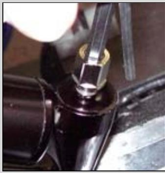
6. If this is an ISX-4, use the special penta-hex tool (P/N 83-3236) to remove the non-adjustable Intrinsic damping assembly. As with the ISX-6, other than the O-rings on the out side of the assembly there are no serviceable parts inside the damping unit so do not attempt to disassemble the unit further
