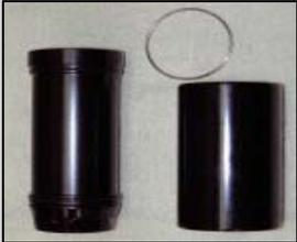
8. If this is a twin-tube Evolver: Remove the snap ring at the base of the can. It is easiest to do this by inserting a small pick into the gap on the ring and lifting one end free of the groove, and then just walk the rest of the ring out. Once the ring is removed, pull the outer can off of the inner can.
