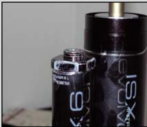
28. Next using a 6mm Allen wrench screw the IFP Positioning tool down to the line matching the travel/stroke of the shock you are servicing, you want the line to just disappear below the top of the flange, see the picture below. You will have oil come out of the damper shaft as you do this. This gives you the final bleed on the shock.
