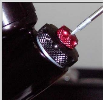
5. If you are servicing an ISX-6, remove the red and black knobs, use caution as the detent balls and springs are VERY small. Next remove the Intrinsic damping assembly by unscrewing it counter clock-wise. Pull the assembly out of the damper body. Do not disassembly the Intrinsic damping unit as there are no serviceable parts inside and several of the parts are easily lost or damaged.
