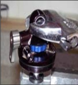
21. Keep the damper shaft pointed straight up and clamp it in the vise with the clamp shafts. Install bottom out bumper and reinstall the top cap using red Loctite. Torque the top cap to 85 inlbs. Note: you may need to turn the Rebound counter clockwise a couple of turns as you are threading the top cap on as it will thread the adjusting needle in due to the detent plate.
