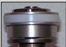
13. If this is an SPV shock, you need to make sure that the SPV valve is functioning correctly. The valve should look like the top picture, with a space between the piston and the top plate and should spring open and closed when the two pieces are squeezed together. If it has failed it will probably look like the second picture and when it is squeezed it will not spring back open.
