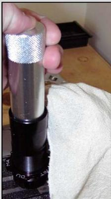
4. Pour out the oil in the damper body. Cover the Reservoir with a rag to catch the IFP and any oil which might be trapped to the reservoir. Insert the IFP removal tool, into the damper body. Cover the hole in the tool with your finger and press the tool down firmly into the damper body. This will push the piston out of the reservoir.
