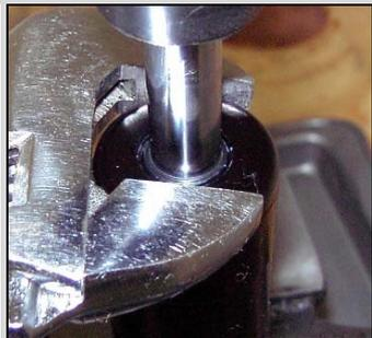
3. Make sure that the shock is full extended. Clamp the shock in a vise by the damper eyelet. Using a 28mm or an adjustable wrench, remove the damper cap and shaft from the shock by turning it counter-clockwise. Drain out as much fluid as possible after pulling the damper assembly out of the shock.
