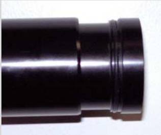
21. If you are servicing an Evolver with a twin tube, grease the two o-rings on the inner can with a small amount of silicone grease. Reinstall the outer can by sliding it on the inner can, be sure that is slid all the way to the end of the inner can.
