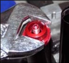
9. Remove the No Tools Volume adjust by unscrewing it counter clockwise. There is no need to disassembly the assembly any further as there are no parts to wear in the no tools adjuster.
