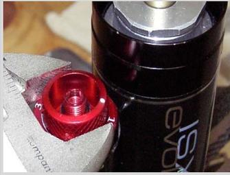
31. Remove the IFP tool from the reservoir and install the Volume control assembly. Torque the assembly to 100inlbs (11Nm). Turn the control to the open position, this is where the indicator is in the number 1 position, this allows the entire volume control to be pressurized. On Swinger X4 shocks charge the IFP to 125psi. For the Evolver shocks the SPV version is charged to 120psi and the shim version to 150psi. The charge pressure is 250psi on the Split shocks.
