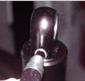
22. Charge the IFP to 125psi using a standard shock pump. Install the small, threaded metal cover over the Schrader valve. You will need to use components from the HP IFP tool kit for this.
