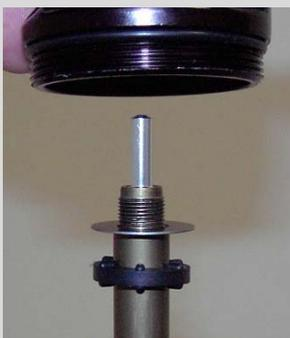
29. Reinstall the rebound needle, bottom out bumper, and the bottom out washer. Clean the tread of all oil residue.
