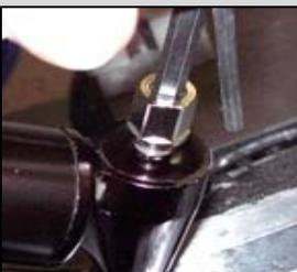
12. If this is an ISX-4, use the special penta-hex tool (P/N 83-3236) to remove the non-adjustable Intrinsic damping assembly. As with the ISX-6, other than the O-rings on the out side of the assy. There are no serviceable parts inside the damping unit so do not attempt to disassemble the unit further.
