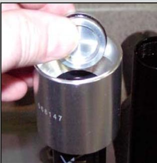
19. Install the bleed bowl, and fill the reservoir and bowl with 5wt shock fluid. Install the IFP by lowering it into the fluid vertically so no air is trapped in the cavity if the piston. Turn the piston 90 degrees and push it into the reservoir past the threads. Remove the oil above the piston. Remove the bleed bowl.
