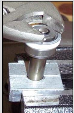
8. To Remove the SPV valve for service, clamp the shaft in the vise using the proper size shaft clamps. Using a \*\*mm wrench loosen the clamp bolt. Remove the bolt, shim stack, piston and the SPV valve. Be sure to keep all items in the proper order and orientation for reassembly.
