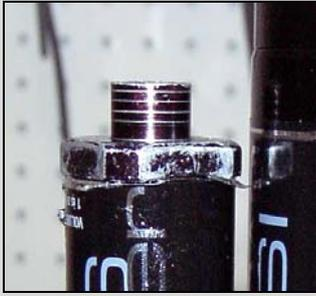
20. Make sure that the IFP Positioning Tool is in its shortest position; Screw it down into the reservoir pushing the IFP into the bore.
