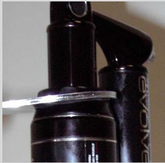
32. Pull the air can up and screw the top cap down. Clamp the top cap in the vise and using a 39mm wrench torque the air can to 80 inlbs ( 9Nm)
