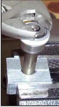
14. To Remove the SPV valve for service, clamp the shaft in the vise using the proper size shaft clamps. Using a \*\*mm wrench loosen the clamp bolt. Remove the bolt, shim stack, piston and the SPV valve. Be sure to keep all items in the proper order and orientation
