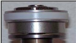
7. If you are working on a shim style shock skip to step #10, if this is an SPV shock, you need to make sure that the SPV valve is functioning correctly. The valve should look like the top picture, with a space between the piston and the top plate and should spring open and closed when the two pieces are squeezed together. If it has failed it will probably look like the second picture and when it is squeezed it will not spring back open.
