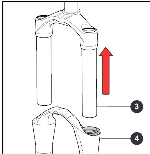
**REMOVING THE HYDRAULIC CARTRIDGE - RIGHT LEG**
