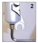
**3.** With hex wrench in shaft bolt, tap right shaft bolt free with plastic mallet. This frees the shaft end from lower leg shaft bore press-fit, and allows lower leg to be removed from upper tubes.
