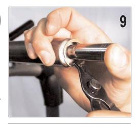
10. Remove wave washer from the Hydra Air/Dual Air side by tipping the fork down to a 45-degree angle. The wave washer will slide down to expose the inner snap ring.
