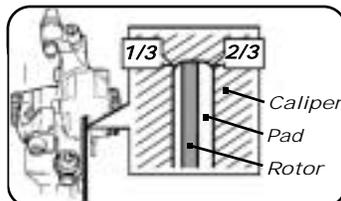
Rotor should be offset to the outboard side of the rotor slot. Ideal ratio is 1/3 to 2/3.
