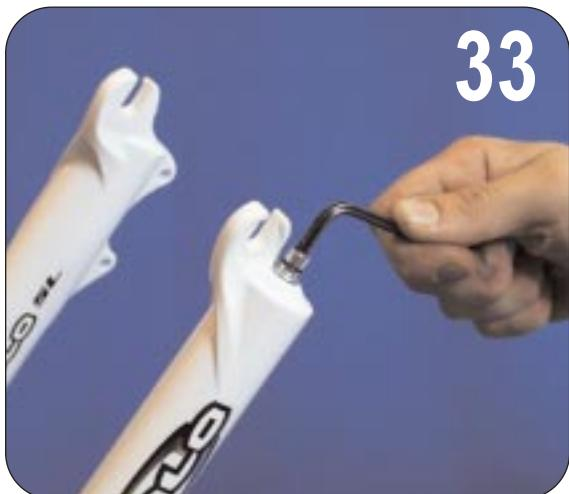
33. Slide the lower legs all the way onto the upper tubes until they engage the shafts.
