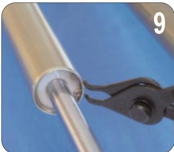
9. Using snap ring pliers, remove the snap ring located underneath the right upper tube.
